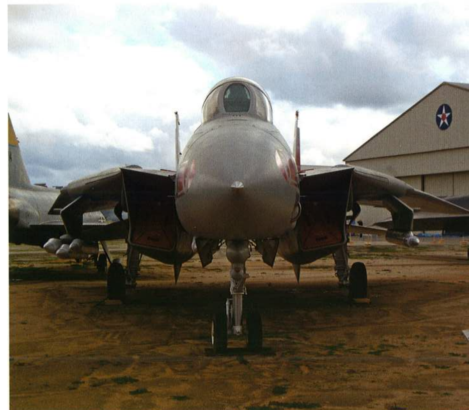
A close up view of the front of YF-14A 157990 at the March Field Museum, showing the right wing fully swept and the left wing further back in the 'superswamp' parked position. Norm deWitt
