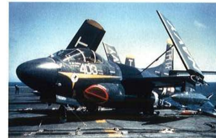
A VF-14 Douglas F3D-2 Skyknight on board the USS Intrepid (CVA-11). This jet night fighter had a short career with the Squadron. Rich Dann
