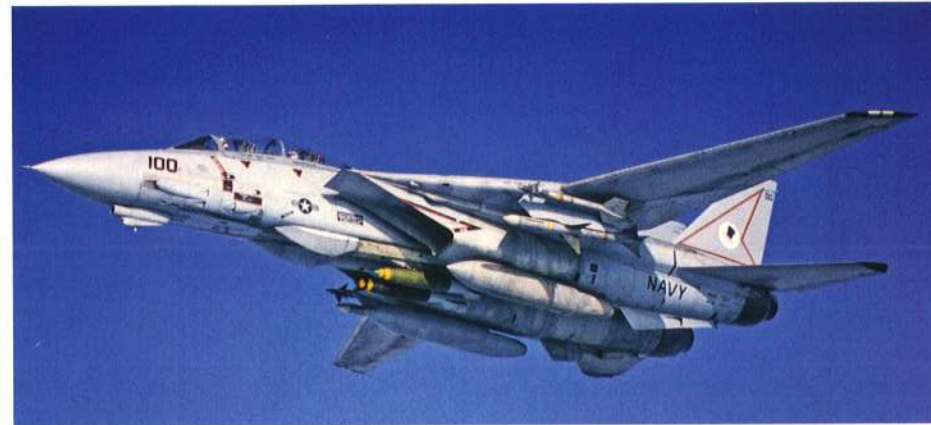
The F-14s of the US Navy were modified to include a ground attack capability. Here a VF-14 Tomcat carries a pair of Mk 84 bombs on the underfuselage forward stations. Rich Dann
