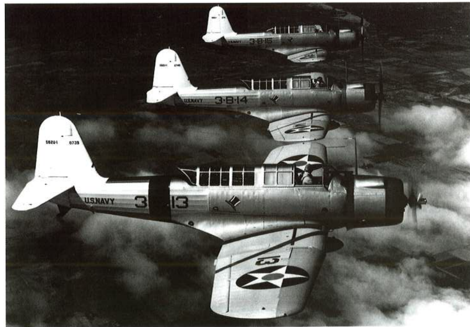
The Vought SB2U Vindicator was a leap forward for US Naval Aviation, its Pratt and Whitney R-1535 825hp engine gave it a maximum speed of 251mph and a ceiling of 27,500 feet. These are SB2U-1s of VB-3. National Museum of Naval Aviation
