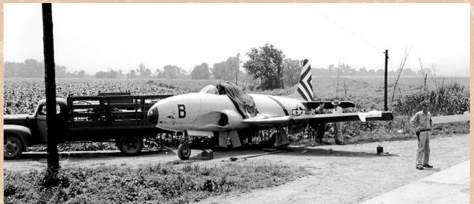
Early engine and fuel pump problems led to some accidents and off airfield landings, as with this early production P-80. USAF
