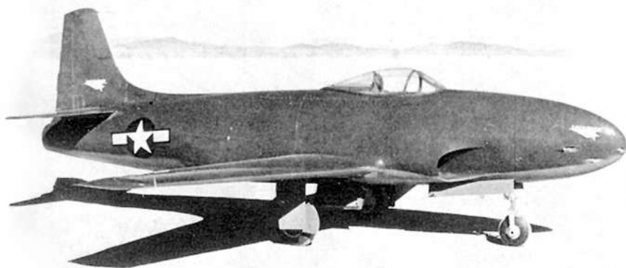
The first XP-80 prototype, Lulu Belle with the early shape of the fin and rudder. This was the only P-80 to be fitted with this design, it was quickly changed to the more rounded fin. USAF
